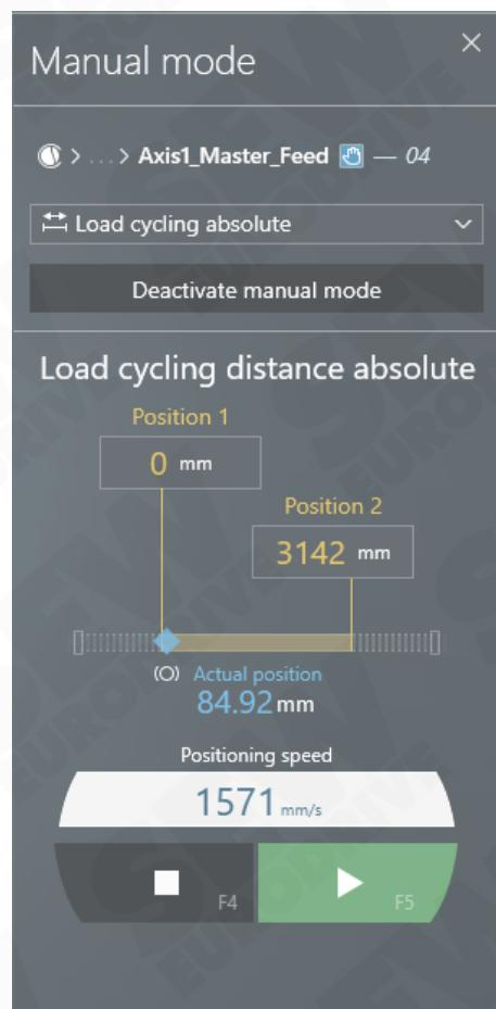
2 To do so, move the axis to the absolute position in manual mode using load cycling
