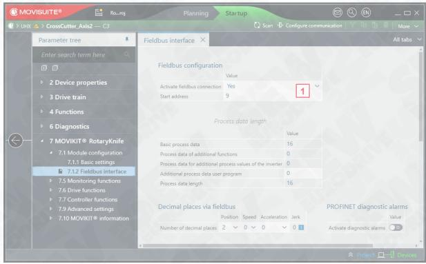
1 Activate the fieldbus connection and set the start address 9.
