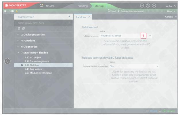
Select the appropriate **Fieldbus protocol**. The fieldbus connection will be automatically activated.
