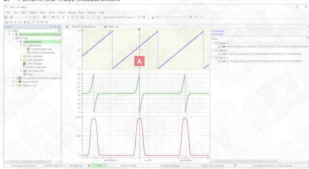
A The cut starts in the middle of the cycle because the rotary knife was at the position of 90° before the master axis started.
