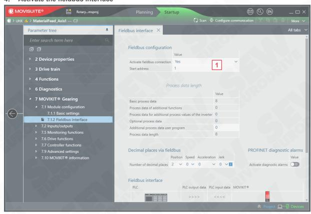
Activate the fieldbus connection and keep the default start address 1
