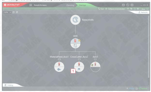
Assign MOVIKIT® RotaryKnife to CrossCutter Axis2 and reset the following error E-34.01 again.
