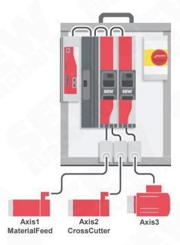
Axis1 / Master **MaterialFeed\_Axis1**: Drive with motor encoder => MOVIKIT® Gearing Axis2 / Slave **CrossCutter\_Axis2**: Drive with motor encoder => MOVIKIT® RotaryKnife Axis3: Drive with motor encoder => not used
