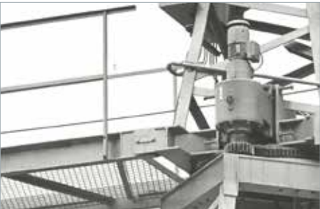
Cranes Slow-turning crane drive, line-powered brakemotor with compound helical gear unit
