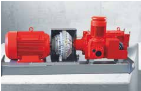
Building materials Bucket elevator drive on joint swing base with main motor, turbo coupling and auxiliary gearmotor
