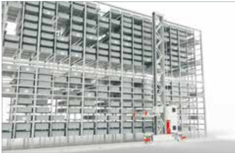
Logistics applications Storage/retrieval system/automated small-parts warehouse
