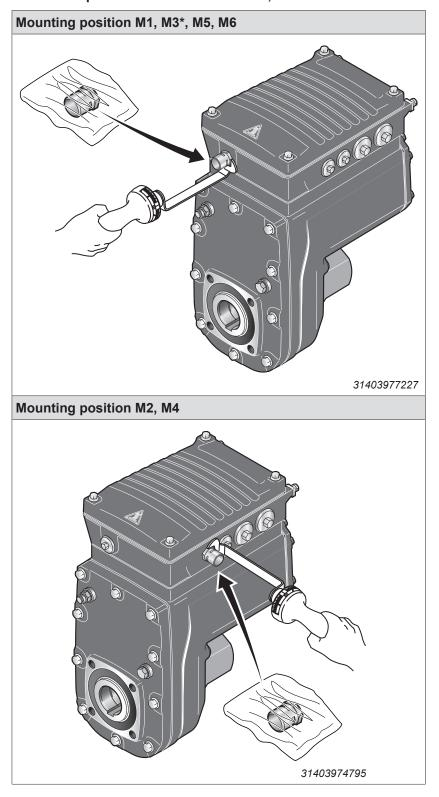
\* Mounting position M3 is only possible with the option "integrated pressure compensation in the gear unit (/PG)".
