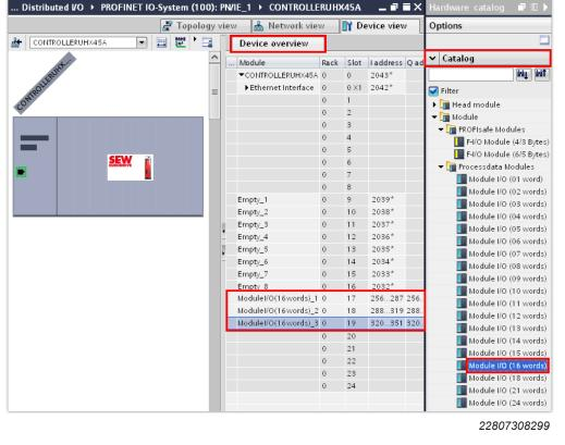
⇒ In this example, 16 process data words are assigned to the each application inverter module (slave of the MOVI-C® CONTROLLER) for communication.
