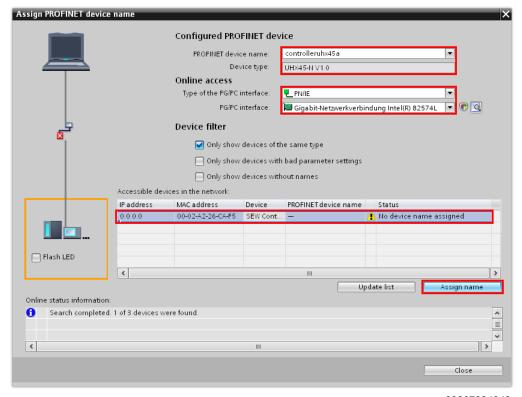
6. Select the PROFINET device name of the MOVI-C® CONTROLLER.
