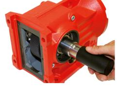
Place the assembly sleeve onto the output shaft.
