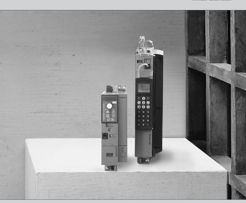
DFE24B and FSE24B EtherCAT® Fieldbus Interface
