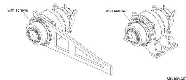
For the following gear unit variants, the screws on the flange side are NOT included in the delivery:
