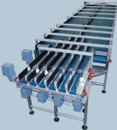
The French company Secma-Cabon offers a comprehensive range of automated plant technology to manufacturers of cans. The systems on offer include a feed table that feeds cans to a sterilizer. The reduction of energy consumption and of the installation effort are very important factors at Secma-Cabon to keep up with the competition in terms of profitability and saved operating costs.
