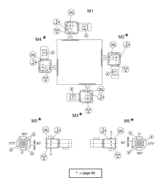
Mounting positions of helical-worm gearmotors
