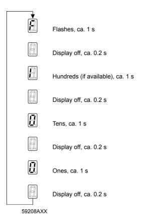
Following a reset or if the error code resumes the value '0', the display switches to the operating display.
