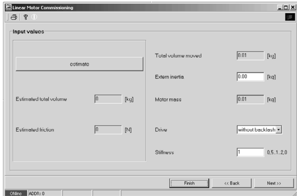
Figure 9: Screen for optimizing the axle using the "Estimate" button and the "Stiffness" input field
