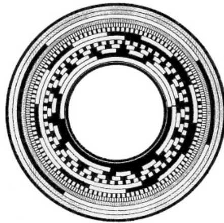
Fig. 52: Code disk with Gray Code
