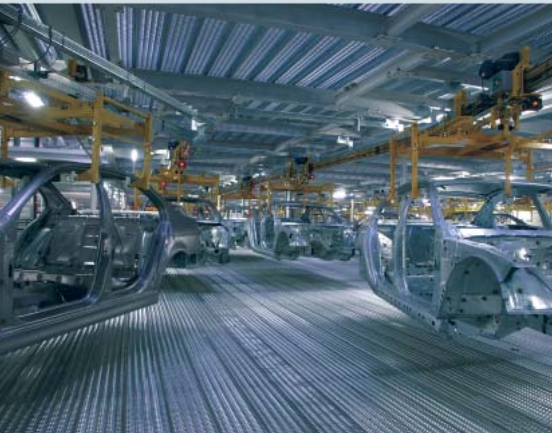
Drives for overhead trolley systems in the automotive industry
