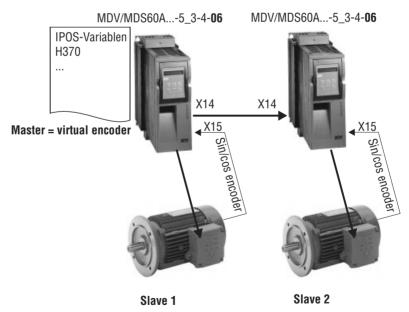
Fig. 3: Master/slave mode with virtual encoder
