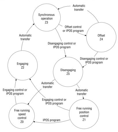
Fig. 1: Overview of the state machine for internal synchronous operation
