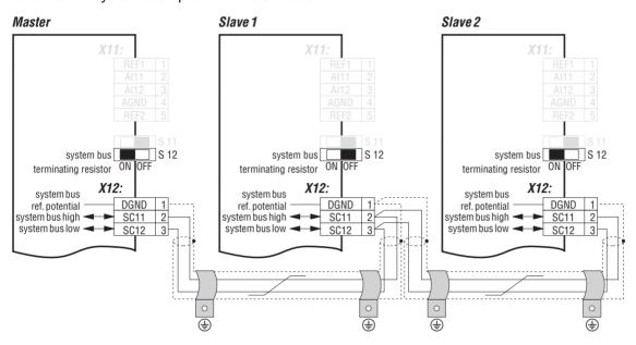
Fig. 11: System bus connection (example: 1 master and 2 slaves)
