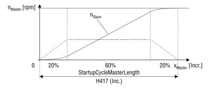
Fig. 15: Speed profile for the travel-dependent synchronization process
