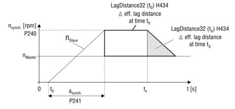
Fig. 14: Speed profile of the time-controlled synchronization process
