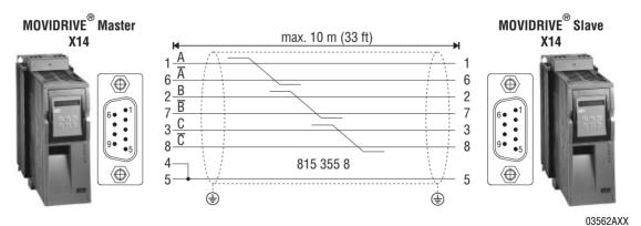
Fig. 10: X14 – X14 master/slave connection
