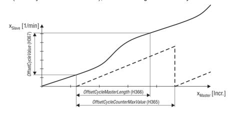
Fig. 24: Position-controlled, travel-dependent offset processing
