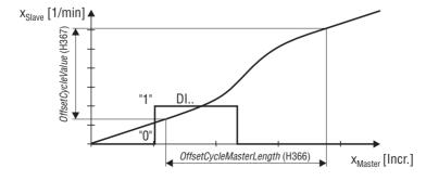
Fig. 23: Travel-dependent offset processing controlled by binary inputs
