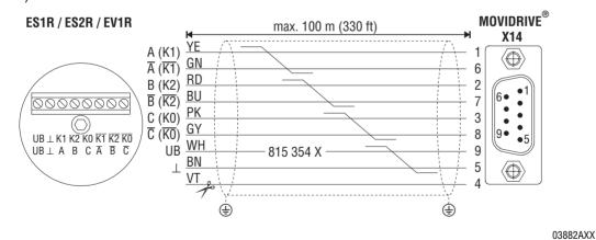
ightharpoonup Cut off the violet conductor (VT) of the cable at the encoder end.
