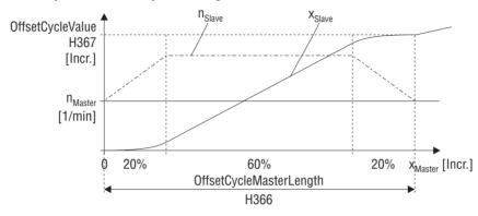
Fig. 22: Speed profile for travel-dependent offset processing
