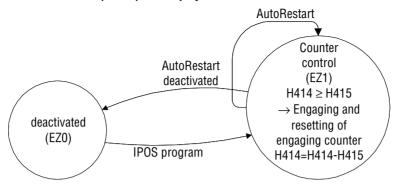
Fig. 20: Startup cycle state machine with position control (engaging mode 3)
