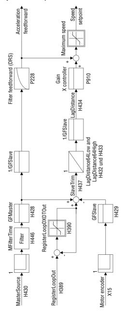
Fig. 26: Block diagram for internal synchronous operation
