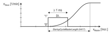
Fig. 16: Event-driven starting of the travel-dependent startup cycle process
