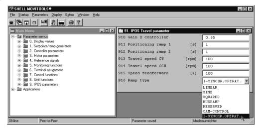
Fig. 12: Activating internal synchronous operation with P916
