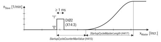
Fig. 17: Interrupt-controlled starting of the travel-dependent startup cycle process
