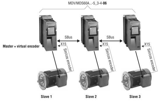
Fig. 5: Group configuration with virtual master encoder
