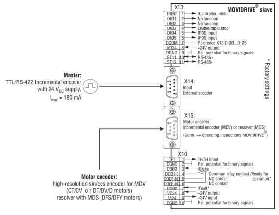
Fig. 7: Connecting the incremental encoder master to MOVIDRIVE® slave
