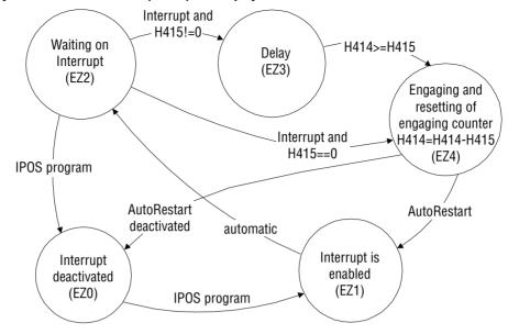
Fig. 18: Startup cycle state machine with interrupt control (engaging mode 2)
