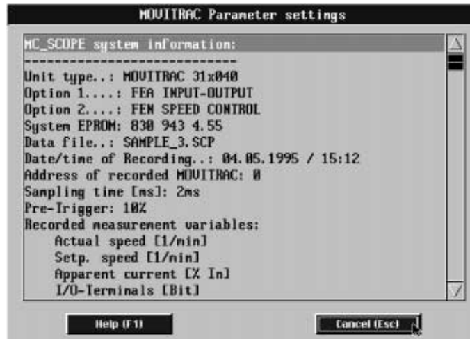
Figure 13: Automatic system documentation by MC_SCOPE
