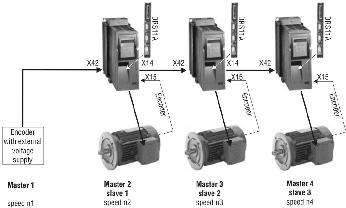
Fig. 4: Master-slave chain with external master incremental encoder
