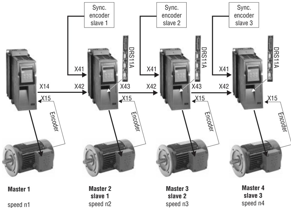
Fig. 5: Master-slave chain with sync. encoder
