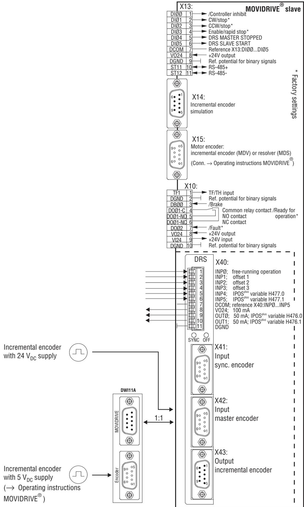
Fig. 11: Incremental encoder master - MOVIDRIVE® slave connection
