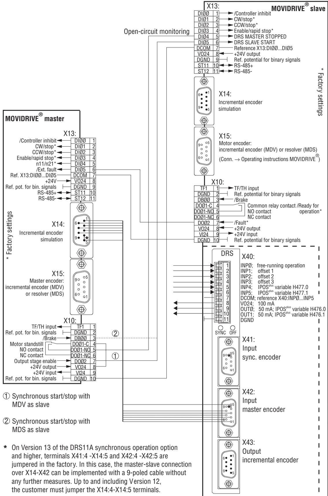
Fig. 9: MOVIDRIVE® master - MOVIDRIVE® slave connection
