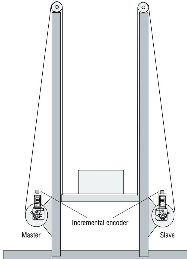
Fig. 12: Two-column hoist
