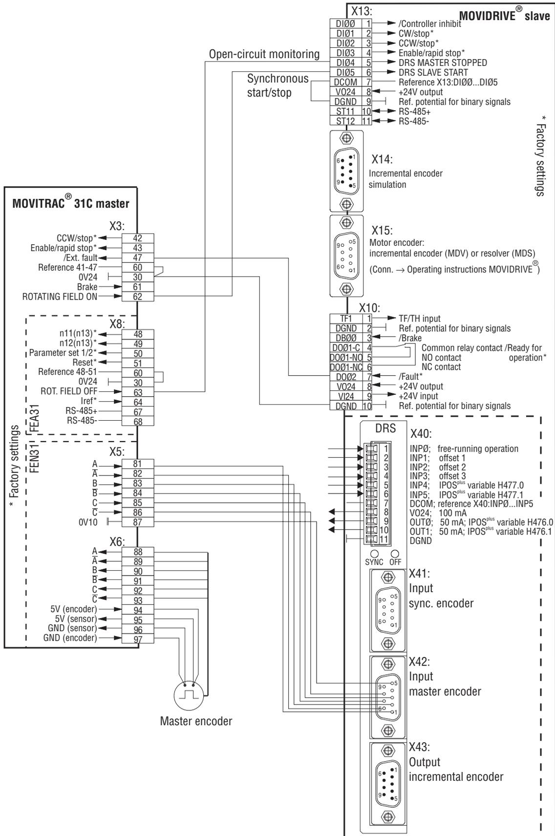
Fig. 10: MOVITRAC® 31C master - MOVIDRIVE® slave connection
