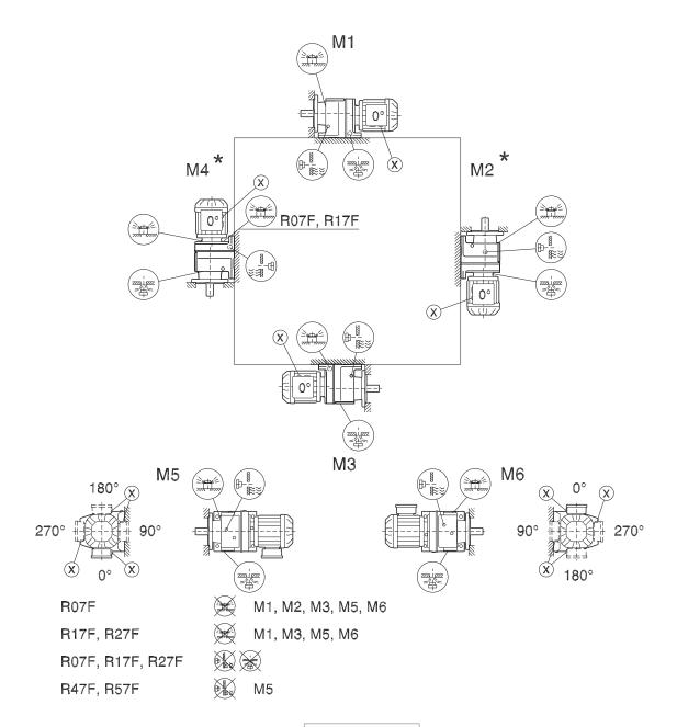
Proper alignment must be ensured when two mounting surfaces are used. Also, the OHL and  $F_{Ra}$  shown in the selection tables is reduced 50% if torque transmission occurs via the mounting flange. ( $\rightarrow$   $\bigcirc$  53)
