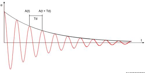
3. Using the "Logarithmic decrement  $\Lambda$ ", calculate the "Decay constant  $\delta$ " and the "Damping factor D" using the following formulae:
