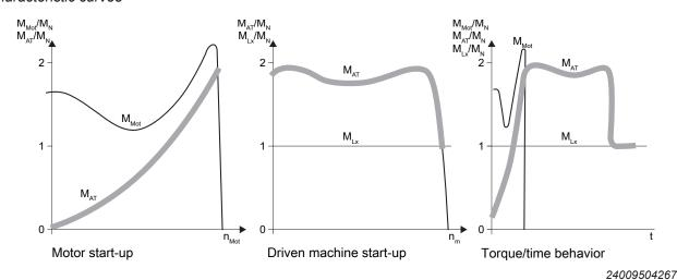
$M_{\text{Mot}}$ Motor torque  $M_N$ Nominal torque  $M_{AT}$ Coupling torque Load torque  $M_{1x}$  $n_{\text{Mot}}$ Motor speed  $n_{m}$
