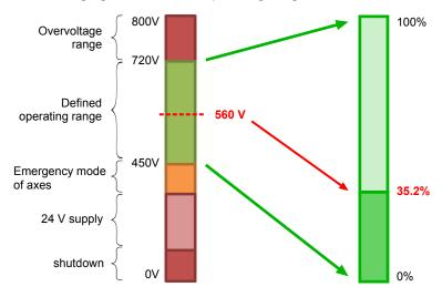
The device operates primarily with the voltage of the DC link or the connected energy storage unit. For the capacitors used, this is an indicator of the amount of charge or energy in the DC link and consequently also of the state of charge.
