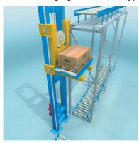
In reverse mode, positioning is performed according to the same principle as for feedin. After positioning in one direction, however, further infeed in the same direction is not possible. Starting another infeed process in the same direction is inhibited by the "In position" signal and prevents unintentional travel to the mechanical stop.
