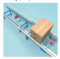
In this roller conveyor, longer track sections are subdivided into segments.
