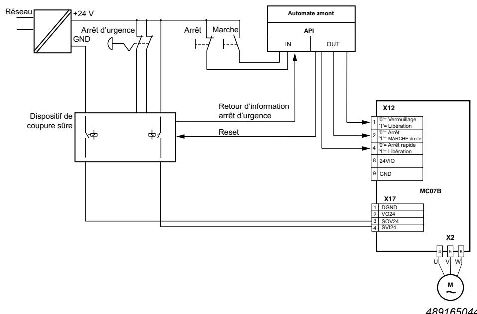
*Pilotage binaire avec dispositif de coupure sûre (un canal)*
