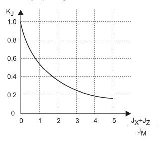
Factor K<sub>M</sub> depending on the external load during run-up
