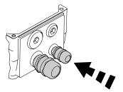
Tighten EMC cable glands supplied by SEW-EURODRIVE using the following torque ratings:
