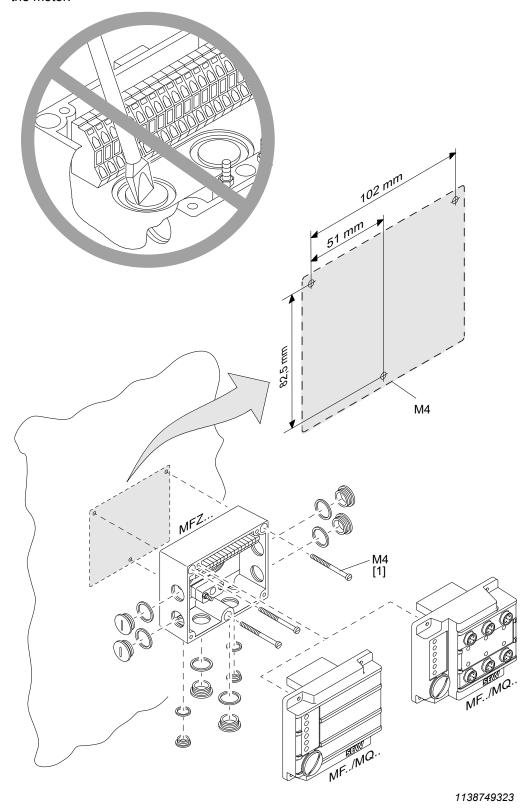
[1] Length of screws min. 40 mm
