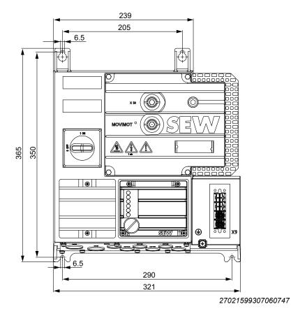
The following figure shows the dimensions of the field distributors MF../MM40/Z.8., MQ../MM40/Z.8.:
