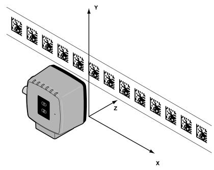
The figure shows the orientation of a read head in the default position of 0°. You can configure the read head for other mounting positions using the interface.
