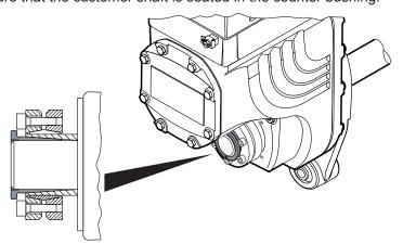
11. Tighten the screws of the shrink disk only hand-tight and ensure that the outer rings of the shrink disk are parallel.
