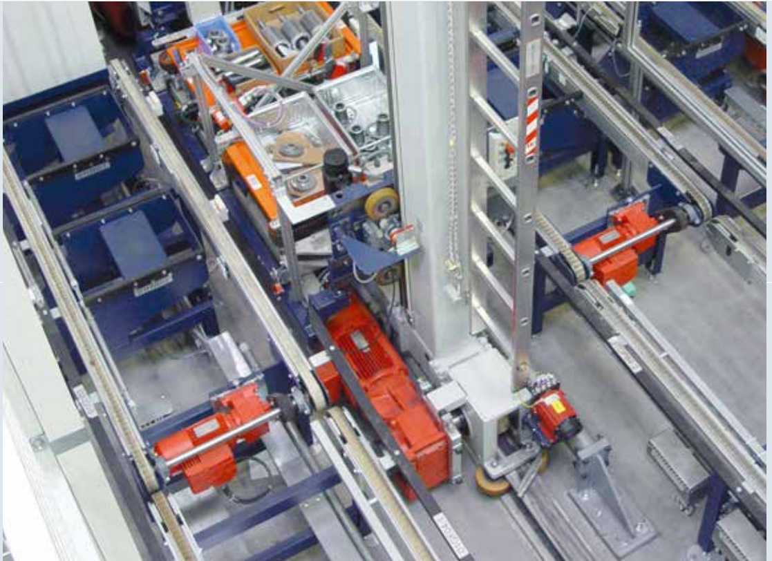
Motor conversion from IE2 to IE3 "made by SEW-EURODRIVE": same weight and same space requirements.
