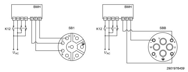
Cut-off in the DC and AC circuits / rapid application of the brake with SBC.
