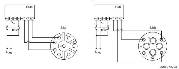
Cut-off in the AC circuit / standard application of the brake with SBC.
