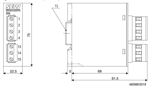
1) Support rail mounting according to EN 50022-35-7.5 (not included in the delivery)
