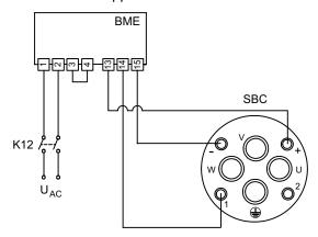
Cut-off in the DC and AC circuits / rapid application of the brake with SB1, SBB.
