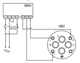
Cut-off in the DC and AC circuits / rapid application of the brake with SBB.
