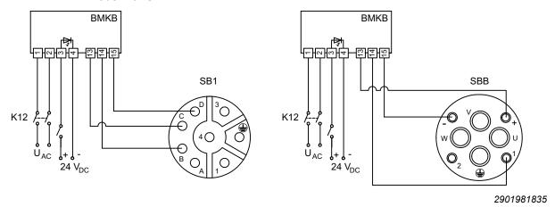
Connection 1, 2 Power supply Connection 3, 4 Signal (inverter)
