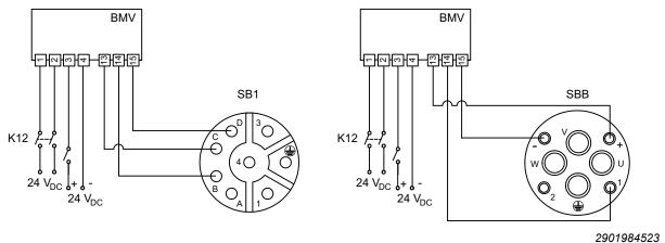
Connection 1, 2 Power supply Connection 3, 4 Signal (inverter) Cut-off in the DC and AC circuits / rapid application of the brake / DC 24 V control input integrated with SBC.
