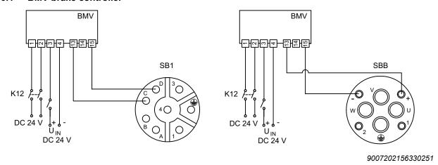
Connection 1, 2 Power supply Connection 3, 4 Signal (inverter)
