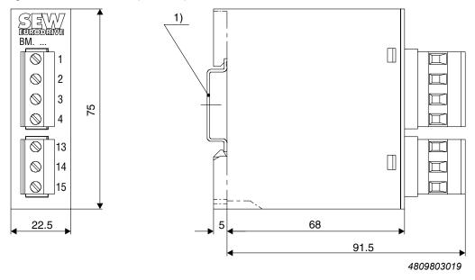
1) Support rail mounting according to EN 50022-35-7.5 (not included in the delivery)
