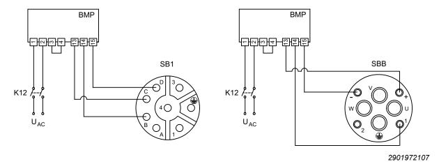
Cut-off in the DC and AC circuits / rapid application of the brake / integrated voltage relay with SBC.
