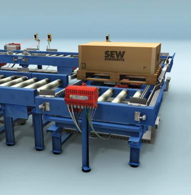
The "universal module" application module is used for speed-controlled and positioning applications. Functional extensions such as synchronization or touch probe evaluation make for a broad range of possible applications.
