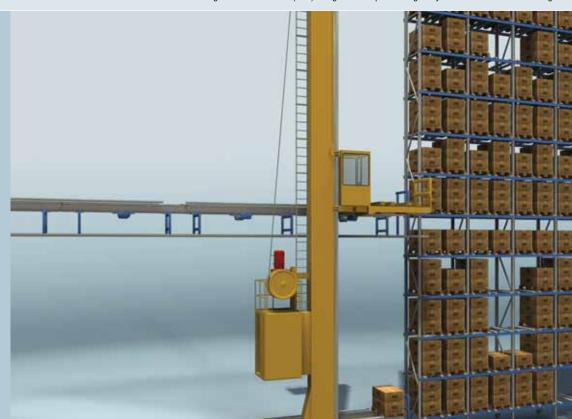
Storage and retrieval unit (SRU) using the example of a high-bay warehouse in warehouse logistics
