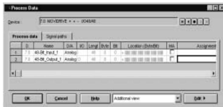
Figure 14: Assigning INTERBUS process data and PLC program addresses
