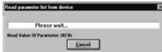
Figure 18: The CMD tool is reading device parameters, i.e. PCP communication is OK.
