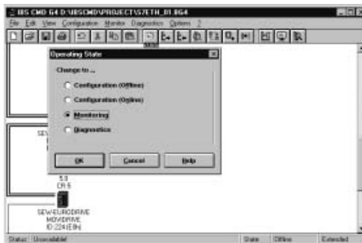
Figure 15: Setting the CMD tool to "MONITORING" operating state
