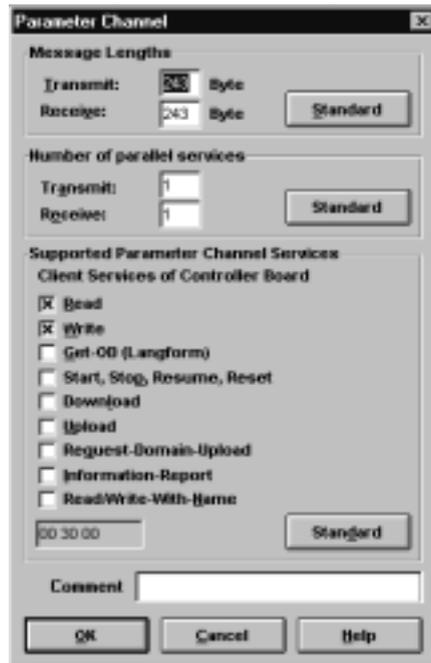
Figure 13: Setting the parameter channel (PCP)
