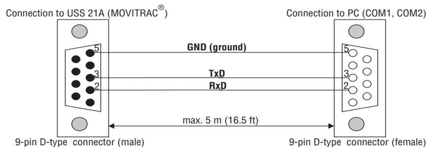
Figure 2: RS-232 connection of MOVITRAC® 31 and PC
