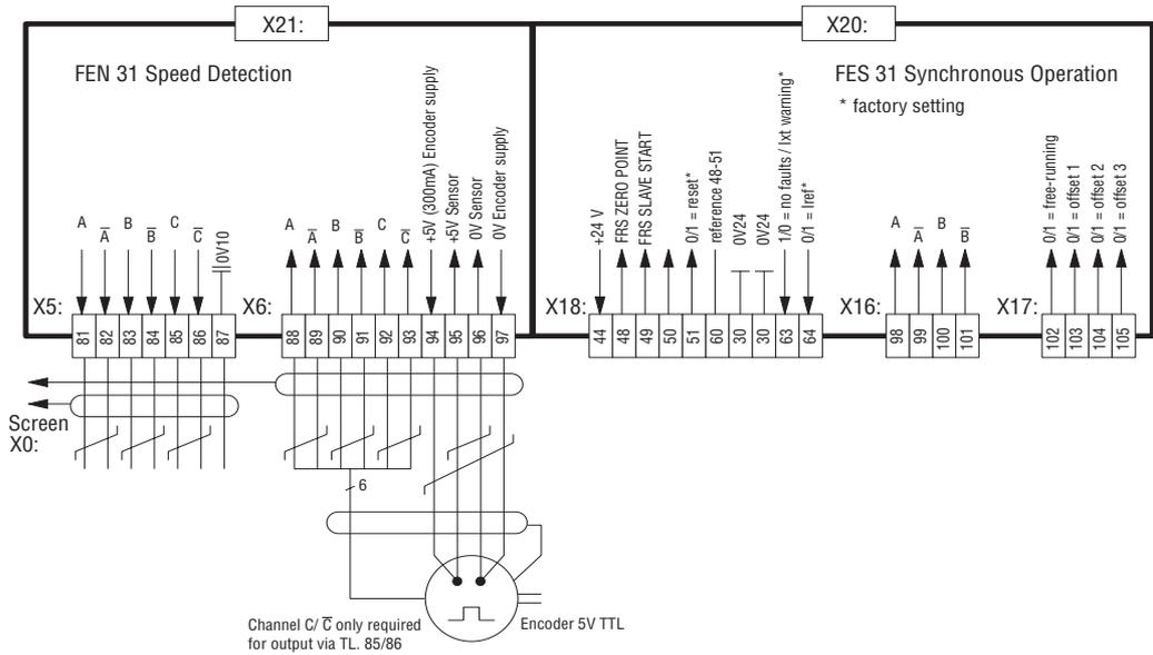
Channel C/  $\bar{C}$  only required for output via TL 85/86
